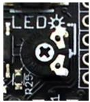
The LEDs on the RCD can be dimmed or brightened by adjusting a trimpot. Use a very small phillips screwdriver (#00 or #000) to adjust the trimpot. Be careful and gentle as you adjust the trimpot. It's safe to adjust the trimpot while the RCD is powered on, but be careful not to touch any components or solder junctions on the board.
