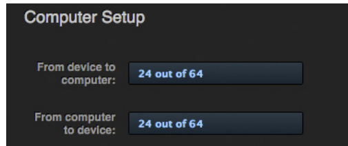
Figure 9-2: The 'From device to computer' setting determines how many channels you see in the Left Input and Right Input menus.
