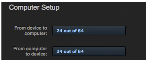
Figure 9-2: The 'From device to computer' setting determines how many channels you see in the Left Input and Right Input menus.
