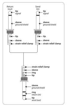
Fig. 4.4: Insert cable with one  $\frac{1}{4}$ " TRS (tip-ring-sleeve) jack plug on one end and two  $\frac{1}{4}$ " TS (tip-sleevel) jack plugs on the other end
