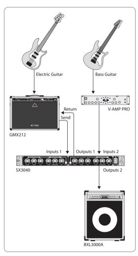
Fig. 3.3: The SX3040 in use with guitar amplifiers
