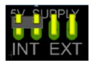
In this setup, no external 5v supply is required Cells will provide 5V from the 12V rail (22mA draw).
