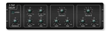
The **3-TAP DELAY** records the input signal and then echoes it back after a user-definable period of time and number of repeats. What makes the stereo and triple delay useful and outstanding is the linked tap-timing and musical choice of echo patterns. Use the 3-TAP DELAY to fatten up vocals and instruments, or to add an enhanced spatial element to any performance.
