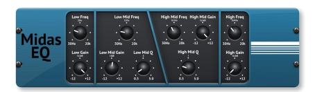
The **4 BAND EQ** is a sweep parametric equalizer, and is taken directly from the MIDAS PRO X Live Digital Console. The bands are low, low mid, high mid and high, with the mid bands using a Q Factor adjustment to custom-tailor the sound. Any combination of the four bands may be used simultaneously.
