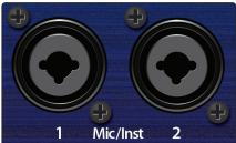
**Microphone/Instrument Inputs.** Both channels of the AudioBox USB96 have Mic/Instrument combo jacks. This convenient connector accepts either a ¼-inch phone plug or an XLR plug.
