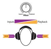
**Power User Tip:** When monitoring your inputs through Studio One or another DAW, it is important that you turn the Mixer knob all the way to the Playback position. Monitoring both the input signal and the playback stream will create a doubling effect that will make monitoring difficult.
