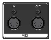
**MIDI I/O.** MIDI stands for "Musical Instrument Digital Interface." MIDI inputs and outputs allow connection to, and communication with, external MIDI equipment. One function of these ports is MIDI sequencing but the MIDI protocol can be used for much more than instruments and sequencing.
