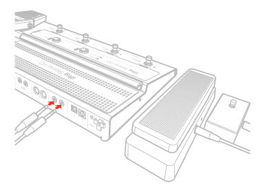
8. If needed, you can connect external MIDI devices to the physical MIDI ports (Input/Output).
