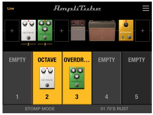
In this mode, the 4 footswitches send MIDI Control Change (CC) messages in order to switch on/off stomps in the AmpliTube path. Changing presets one by one is also possible by holding footswitch 1 or 2.
