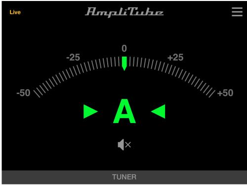
When iRig Stomp I/O is in tuner mode the footswitche's LEDs show the tuning status.
