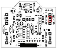
There is a jumper connector installed across two pins here. Removing the jumper disengages the tone control (LIFE).
