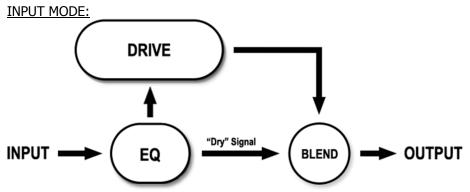
In INPUT mode the EQ comes first in the signal path, affecting both the clean signal and the signal fed into the distortion. Boosting frequencies in this mode can help drive the distortion signal to a more saturated tone.
