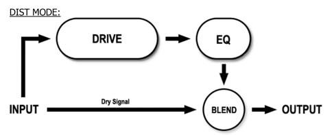
In DIST mode the EQ comes after the distortion signal, having a strong effect on the sound of the distorted signal. The clean signal is not affected by the EQ at all.
