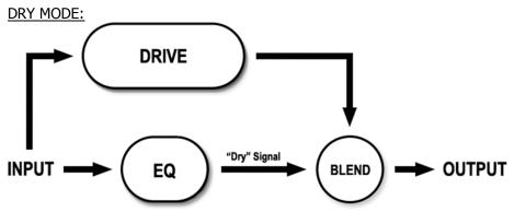
In DRY mode the EQ affects the clean signal, but doesn't affect the distorted signal at all.
