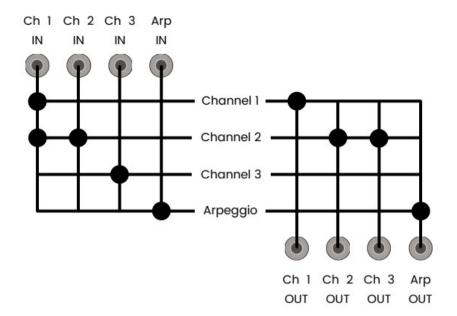
Now let's look at how channel 2 operates here: The pitch that is read at channel 1's IN jack is being **added** to that of Channel 2's IN jack. The resulting input pitch is then quantized through Channel 2. The resulting output pitch of Channel 2 is output not only on Channel 2's OUT jack but also at Channel 3's OUT jack.
