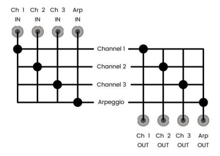
The pitch input of the IN jack of channel 1 is being sent to channel 1, quantized there and output at the OUT jack of channel 1. Not very surprising.
