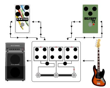
In the example above, mixing two very different overdrives on bass, in parallel, can result in a very full and unique distorted bass tone. You can also use the built in DRY blend on the Tri Parallel Mixer to retain some of the bass guitar's natural low end.
