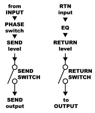
All three channels are setup this way. By default, when a given channel is active both the SEND SWITCH and RETURN SWITCH are closed, allowing signal to flow through them. When a given channel is inactive, both of these switches are open, blocking any signal from flowing. Advance options allow you to change how this works, expanding the Tri Parallel Mixer's possible applications.
