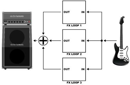
Use the CH 1/2/3 footswitches to activate their respective effects loops. Double tap any of these footswitches to enter master bypass, which connects the INPUT jack directly the OUTPUT jack. When in bypass, single tap any footswitch to re-enter active mode. There are other switching options and configuration options that will be discussed later in this manual.
