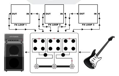
In this configuration, plug your guitar or other instrument/sound source into the INPUT jack on the right of the Tri Parallel Mixer. Connect your amplifier or other sound destination to the OUTPUT jack on the left of the Tri Parallel Mixer. All connections can be made using standard <sup>1</sup>/<sub>4</sub>" instrument cables.
