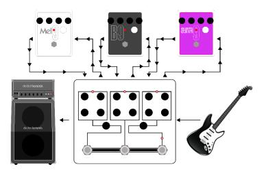
In the example above, you can use three separate effects from the EHX 9 Series, in this case a Mel9 Tape Replay Machine, B9 Organ Machine, and Synth9 Synthesizer Machine, and combine them in parallel to create a mix of mellotron, organ, synthesizer, and guitar tone.
