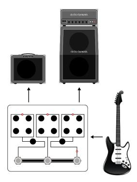
**Figure 1:** An example where you may make use of RETURN MUTING mode. Even when channel one is inactive, bass guitar signal will still flow out of the SEND 1 jack and into the EHX Battalion Bass Preamp/DI. This allows the signal to always come out of the Battalion's XLR out, but only when the channel is active would it be routed to the amp.
