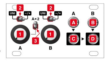
then be inverted with the polarity switch and scaled with Channel A's attenuator knob.
