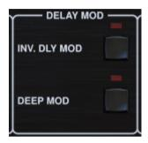
When engaged, the INV DLY MOD button inverts the flanger sweep start and the envelope pitchshift direction. This only applies to Delay Mod Waveforms ENV and TRIG.
