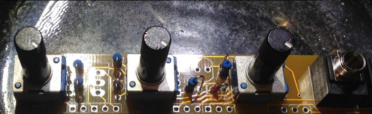
insert switch, make sure you put one nut on the switch before the panel goes on. insert the led, pay attention to polarity. the flat side should face down. the led must be a bicolor two pin.
