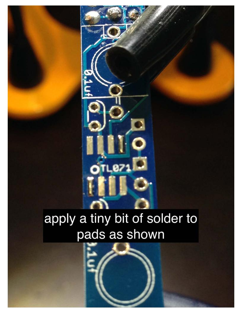
paying attention to chip orientation hold the ic down with tweezers and solder ONE of the previously tinned pads to the leg enusring the leads line up with the pads and the chip is relatively flat. you might have to repeat this process until the chip is lined up properly. then solder the diagonal tinned pad to the leg to lock the chip in place.
