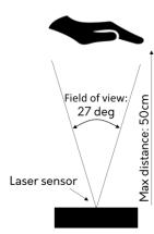
Lazer measures the distance between your hand and its sensor, and it transforms it into analog (gate/cv), MIDI (DIN and USB) and audio signals. The blue led intensity is proportional to the controlled parameter and it blinks when your hand is beyond the configured **Distance range**. The red led turns on if your hand is within the configured **Distance range**.
